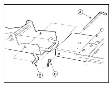
Figure 18. Removing Snow Blade from Hitch
